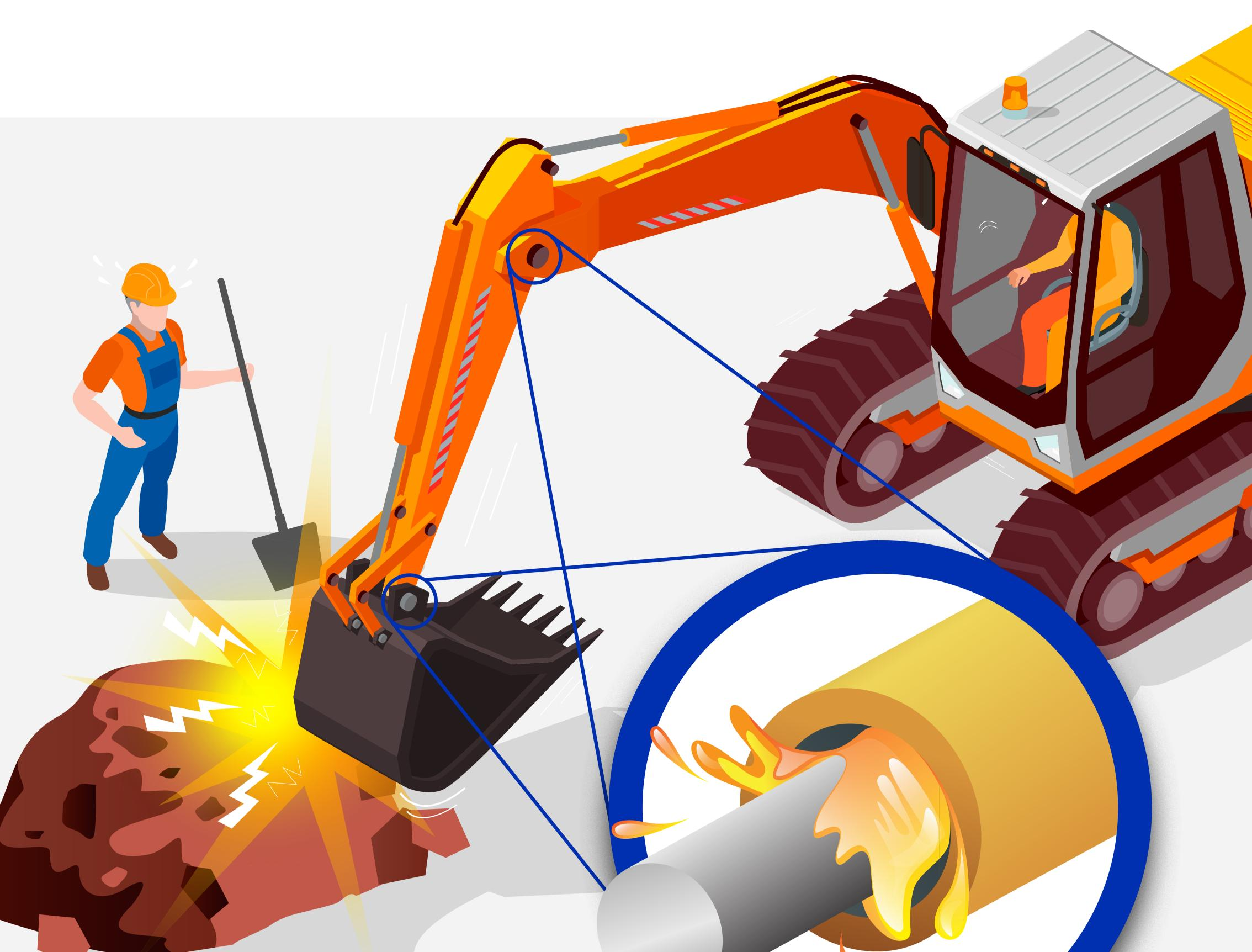
With every hit the grease between the pin and bushing is squeezed out, creating metal-to-metal contact
